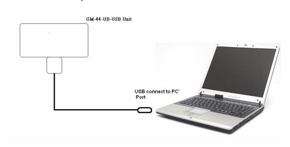
Hardware Requirement: Computer 486 or Faster CPU, VGA Display card, Sound board (optional), at least 16MB DRAM, CD-ROM drive, Windows OS, at least a USB port available.
